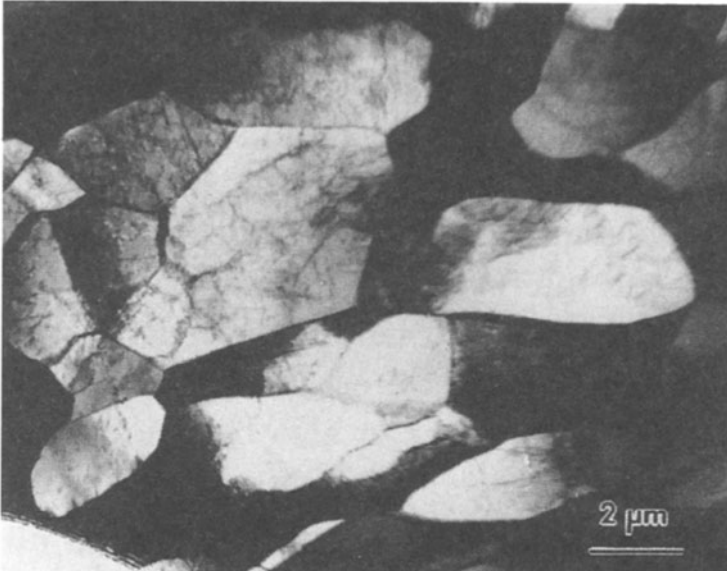
Figure 16.1. TEM-micrograph (X5700) of Silicon-Steel. Reprinted from Axelrad, D. R. (1993) Stochastic Mechanics of Discrete Media , Springer-Verlag Berlin Heidelberg, pp. 64, with kind permission from Springer-Verlag Berlin Heidelberg.
